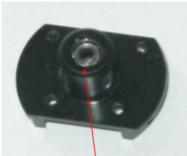
Ballrace seats in the rebate and bottoms on the outer flange.
